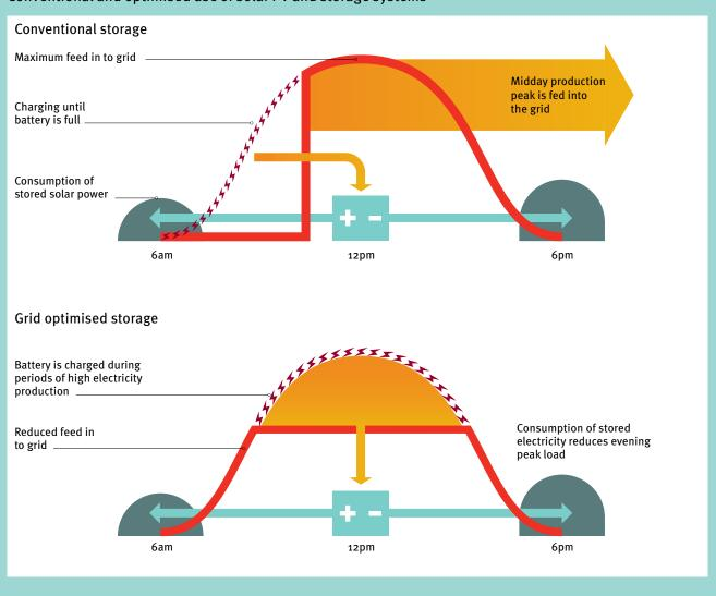
Conventional and optimised use of solar PV and storage systems<sup>44</sup>
